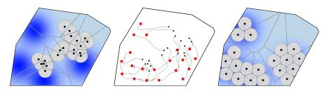
Figure 5.4 Evolution of  $(S_{LD}, Lmtd-Vrn-NrmL)$  with n=20 robots and r=0.4. The left (respectively, right) figure illustrates the initial (respectively, final) locations and Voronoi partition. The central figure illustrates the evolution of the robots. The  $\frac{r}{2}$ -limited Voronoi cell of each robot is plotted in light gray. After 36 seconds, the value of the multicenter function  $\mathcal{H}_{area,\frac{r}{2}}$  is approximately 14.141.
