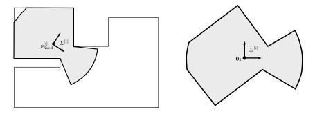
Figure 3.8 The left plot depicts the range-limited visibility set  $Vi_{disk}(p_{fixed}^{[i]}; Q)$  expressed with respect to an inertially fixed frame. The right plot depicts the range-limited visibility set expressed with respect to the body-fixed frame  $\Sigma^{[i]}$ , that is,  $Vi_{disk}(\mathbf{0}_2; Q_i)$ .
