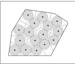
Figure 5.8 Evolution of  $(S_D, VRN-NCNTR)$  with n=16 robots. The left (respectively, right) figure illustrates the initial (respectively, final) locations and Voronoi partition. The central figure illustrates the evolution of the robots. After 20 seconds, the value of the multicenter function  $\mathcal{H}_{sp}$  has monotonically increased to approximately 0.2498 meters.
