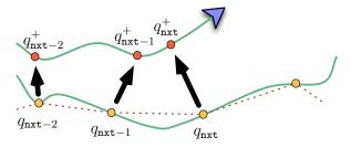
Figure 6.6 Projection of interpolation point  $q_{nxt}$  onto the curve path.
