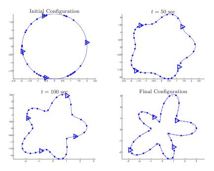
Figure 6.10 Approximate Estimate and Balancing Law for a time-varying boundary: configuration of agents (drawn as triangles) and interpolation points at time instants 0, 50, 100, 200. The last figure shows also the approximating polygon.
