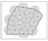
Figure 5.7 Evolution of ( $S_D$ , VRN-CRCMCNTR) with n=16 robots. The left (respectively, right) figure illustrates the initial (respectively, final) locations and Voronoi partition. The central figure illustrates the evolution of the robots. After 20 seconds, the value of the multicenter function  $\mathcal{H}_{dc}$  has monotonically decreased to approximately 0.43273 meters.
