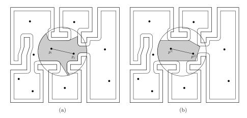
Figure 4.3 The plot in (a) shows the set  $\operatorname{Vi}_{\operatorname{disk}}(p^{[i]};Q_\delta)\cap \overline{B}(\frac{1}{2}(p^{[i]}+p^{[j]}),\frac{r}{2})$ . The plot in (b) shows the outcome of the execution of the ITERATED TRUNCATION ALGORITHM. Robots i and j are constrained to remain inside the shaded region in (b), which is a convex subset of  $Q_\delta$  and of the closed ball with center  $\frac{1}{2}(p^{[i]}+p^{[j]})$  and radius  $\frac{r}{2}$ .
