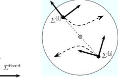
Figure 4.1 Illustration of the connectivity maintenance constraint. Starting from positions  $p^{[i]}$  and  $p^{[j]}$ , the robots are restricted to move inside the disk centered at  $\mathcal{X}_{\mathrm{disk}}(p^{[i]},p^{[j]})=\frac{1}{2}\big(p^{[i]}+p^{[j]}\big)$  with radius  $\frac{r}{2}$ .
