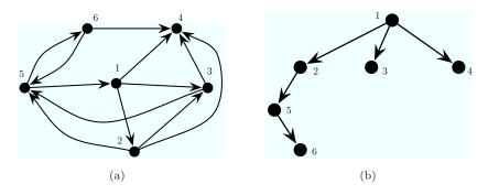
Figure 1.15 Example execution of the Flooding algorithm. The source is vertex 1. (a) shows the network and (b) shows the BFS tree that results from the execution.
