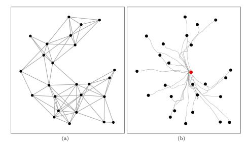
Figure 4.11 Evolution of  $(S_{\infty\text{-disk}}, \text{PLL-CRCMCNTR})$  with n=25 robots in 2 dimensions. (a) shows the initial connected network configuration and (b) shows the evolution of the individual agents until rendezvous is achieved.
