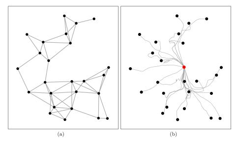
Figure 4.8 Evolution of ( $S_{disk}$ , CIRCUMCENTER) with n=25 robots in 2 dimensions. (a) shows the initial connected network configuration and (b) shows the evolution of the individual agents until rendezvous is achieved.
