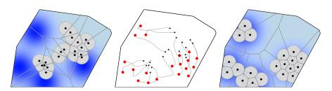
Figure 5.5 Evolution of ( $\mathcal{S}_{LD}$ , LMTD-VRN-CNTRD) with n=20 robots and r=0.4. The left (respectively, right) figure illustrates the initial (respectively, final) locations and Voronoi partition. The central figure illustrates the evolution of the robots. The  $\frac{r}{2}$ -limited Voronoi cell of each robot is plotted in light gray. After 90 seconds, the value of the multicenter function  $\mathcal{H}_{\text{distor-area},\frac{r}{2}}$  is approximately -.386.
