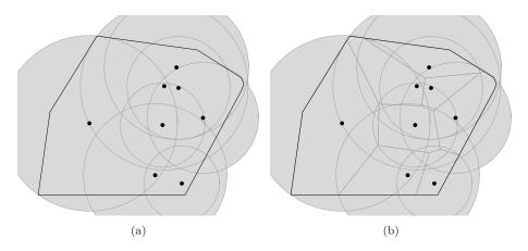
Figure 2.13 Illustration of the definition of  $\mathcal{H}_{dc}$ . (a) and (b) show the same configuration, with and without the Voronoi configuration, respectively. For each node, the disk is the minimum-radius disk centered at the node and enclosing the Voronoi cell. The value of  $\mathcal{H}_{dc}$  is the radius of the disk centered at the leftmost node.
