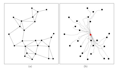
Figure 4.10 Evolution of  $(S_{LD}, CIRCUMCENTER)$  with n=25 robots in 2 dimensions. (a) shows the initial connected network configuration and (b) shows the evolution of the individual agents until rendezvous is achieved.
