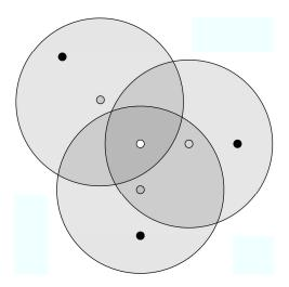
Figure 4.2 Illustration of network connectivity maintenance. The connectivity  $\mathcal{X}_{\rm disk}$ -constraint set of the white-colored agent is the intersection of the individual constraint sets determined by its neighbors.
