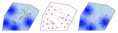
Figure 5.2 Evolution of  $(S_D, VRN-CNTRD)$  with n=20 robots. The left (respectively, right) figure illustrates the initial (respectively, final) locations and Voronoi partition. The central figure illustrates the evolution of the robots. After 13 seconds, the value of the multicenter function  $\mathcal{H}_{distor}$  has monotonically increased to approximately -.515.
