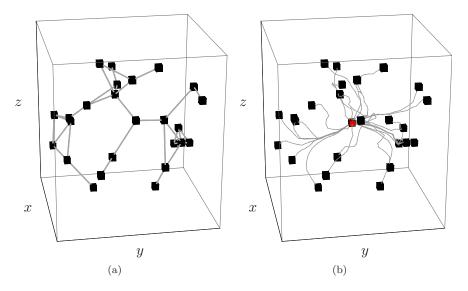
Figure 4.9 Evolution of ( $\mathcal{S}_{\text{disk}}$ , CIRCUMCENTER) with n=25 robots in 3 dimensions. (a) shows the initial connected network configuration and (b) shows the evolution of the individual agents until rendezvous is achieved.
