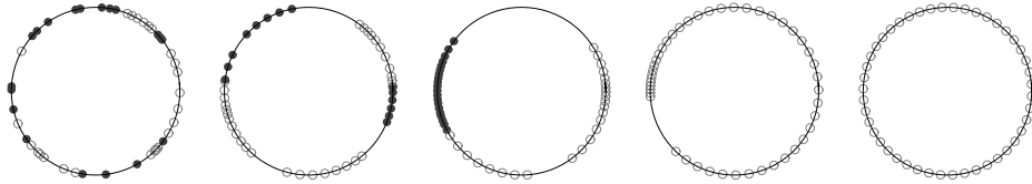
Figure 3.4 The AGREE & PURSUE law. Red-colored disks and blue-colored circles correspond to robots moving counterclockwise and clockwise, respectively. The initial positions and the initial directions of motion are randomly generated. The five diagrams depict the state of the network at times 0, 9, 20, 100, and 800.
